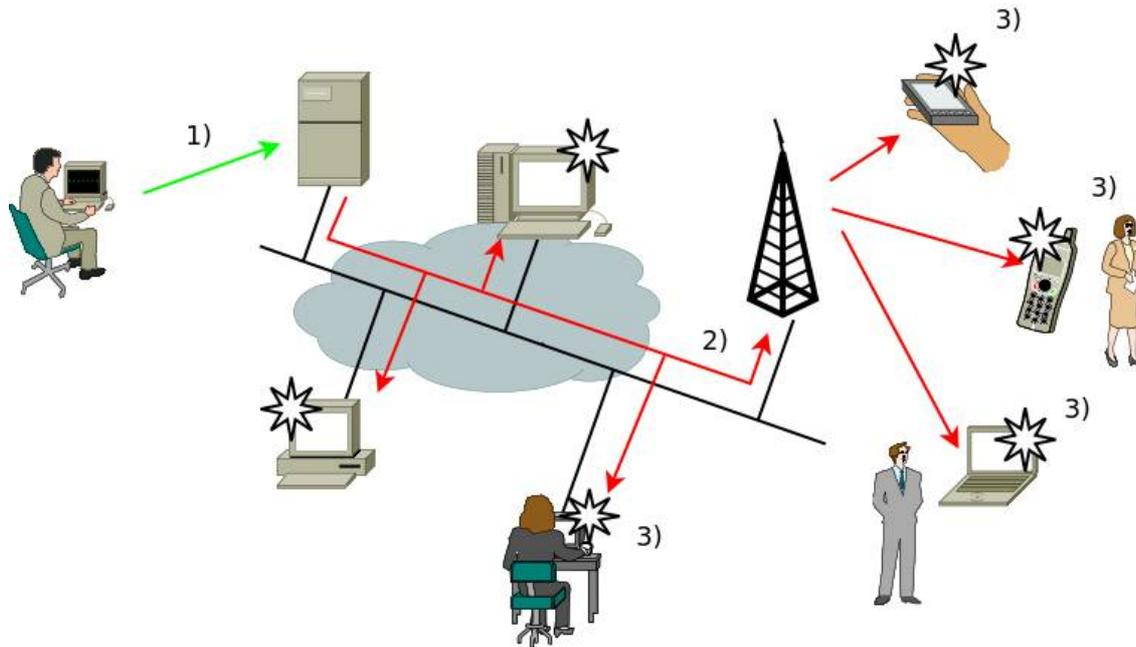
**Figure 1. The administrator publish a news on the server (1) and the message is then sent to the appropriate IPv6 multicast group (2); when the devices joined to the group receive the updated feed, an alert is shown and users are quickly informed.**
